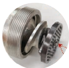
ASSEMBLE ORDER: WORM, KNIFE AND PLATE
